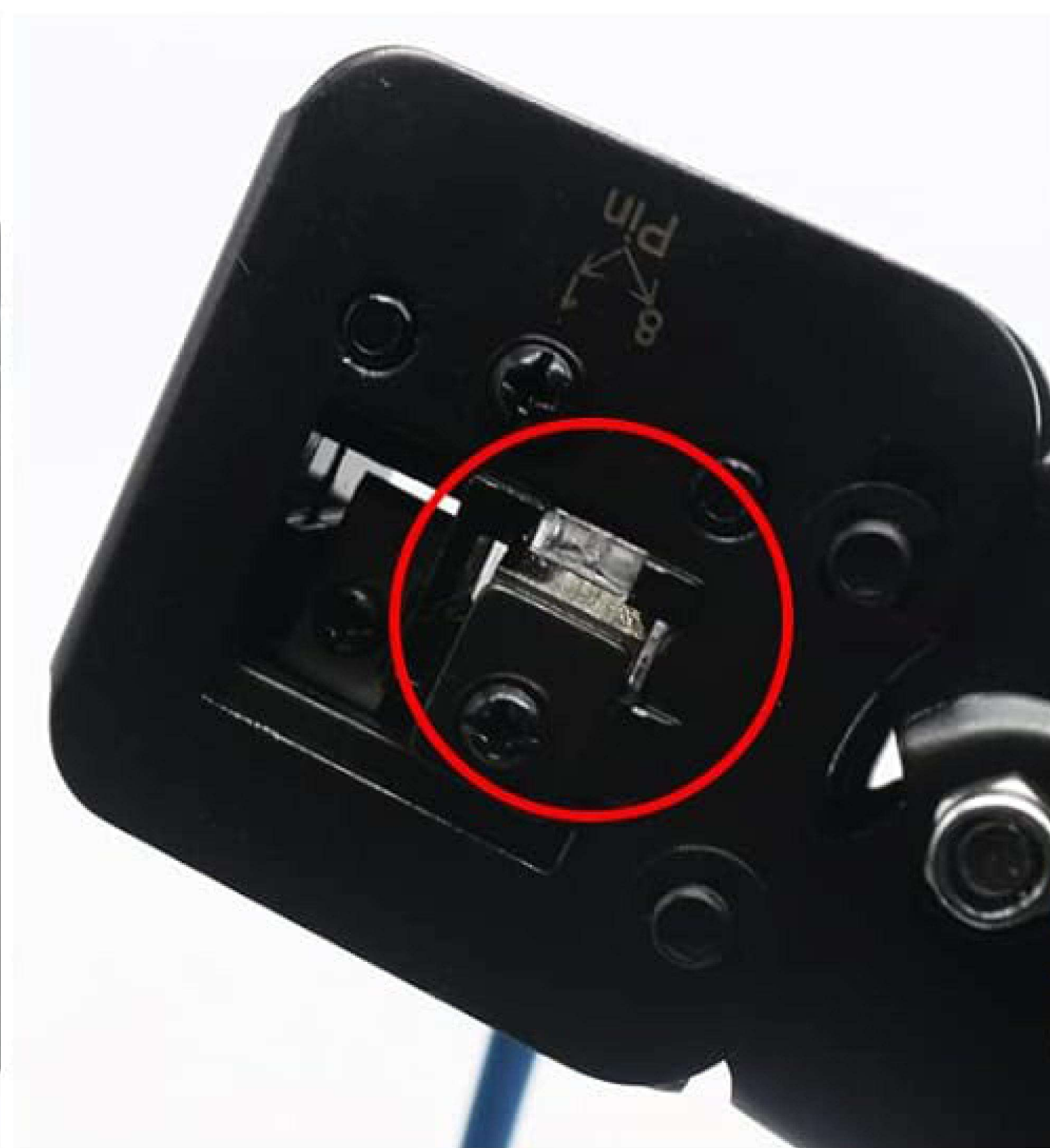
5. After aligning the network cable pliers with the crystal head neatly, press down firmly
