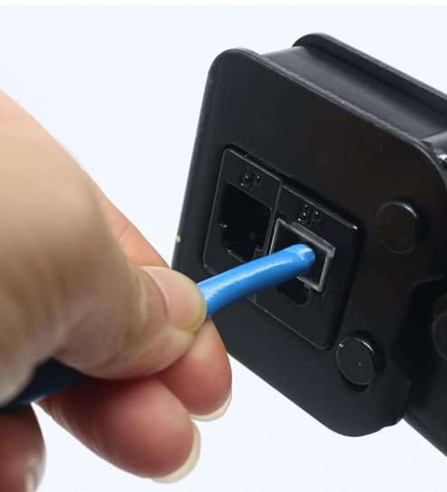
4. Put the crystal head with the network cable into the cable clamp inside the crimping port
