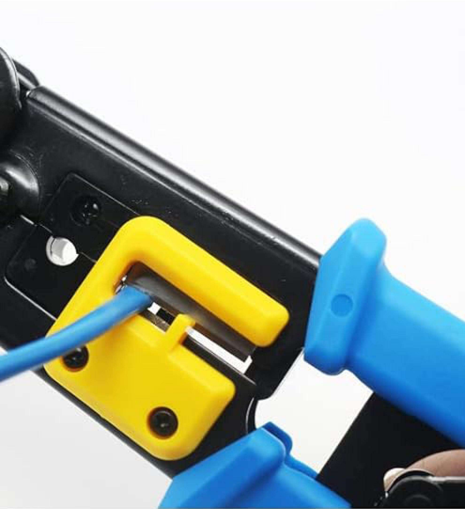
1. Use wire cutters to cut the shell of the network cable
